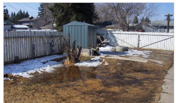
Low areas in the yard can result in pooling and flooding during heavy rain or snow melt
