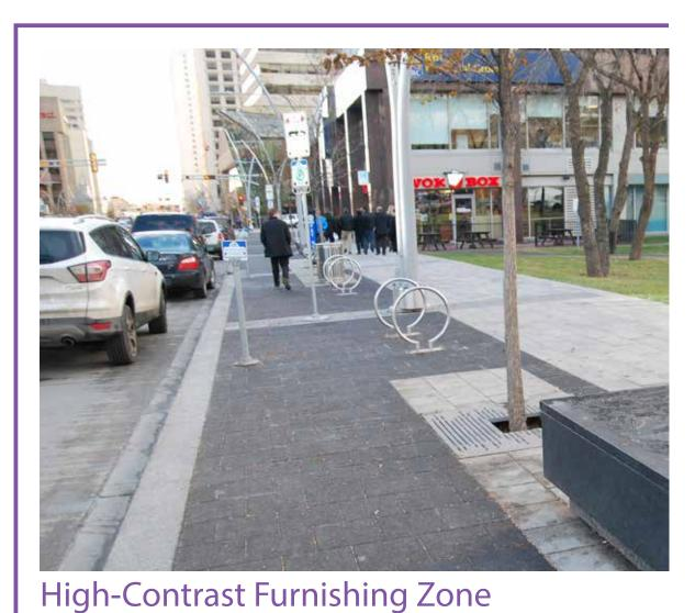
Contrasting colour of paving in the furnishing zone improves wayfinding clarity for the visually impaired. Dark colour concrete paving stones, similar to Jasper Avenue New Vision are proposed.
