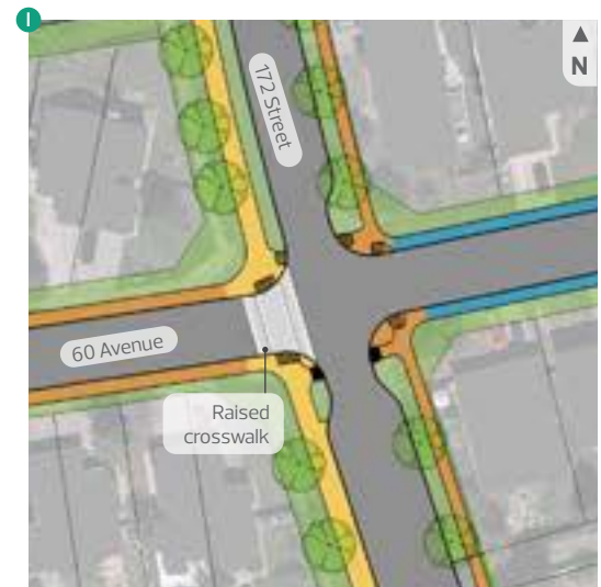
Figure 15. Intersection redesign (172 Street and 60 Avenue)
