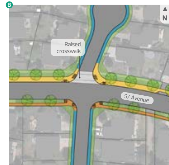
Figure 8. Intersection redesign (57 Avenue and 57 Avenue Cul-de-sac 2)
