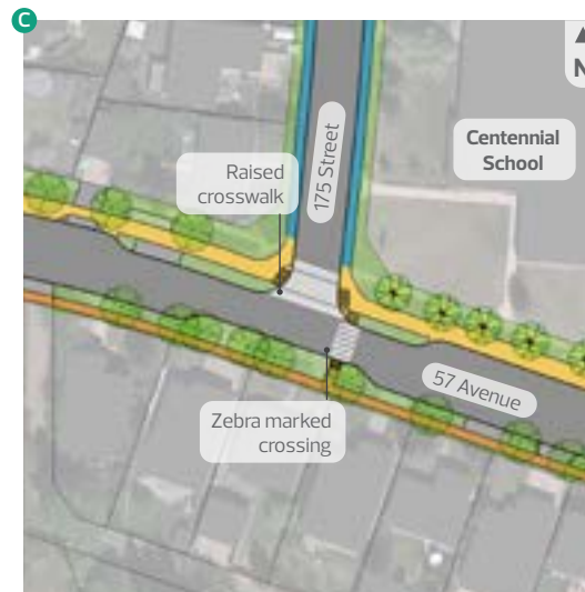
Figure 9. Intersection redesign (57 Avenue and 175 Street)
