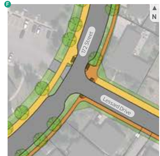
Figure 12. Intersection redesign (172 Street and Lessard Drive)
