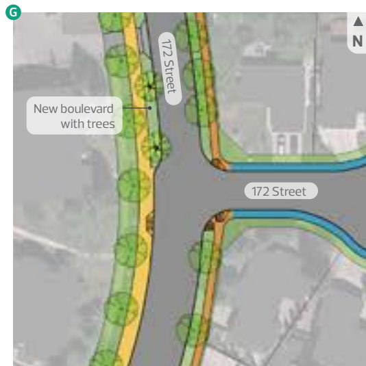
Figure 13. Intersection redesign (172 Street and 172 Street Cul-de-sac)
