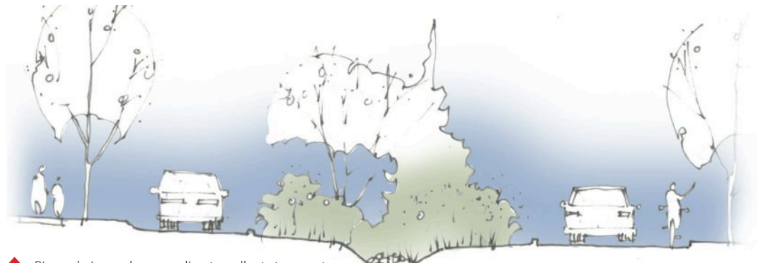
▲ Bioswale in roadway median to collect stormwater.
