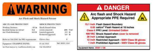
Figure 1 – Examples of Arc Flash & Shock Hazard Labels
