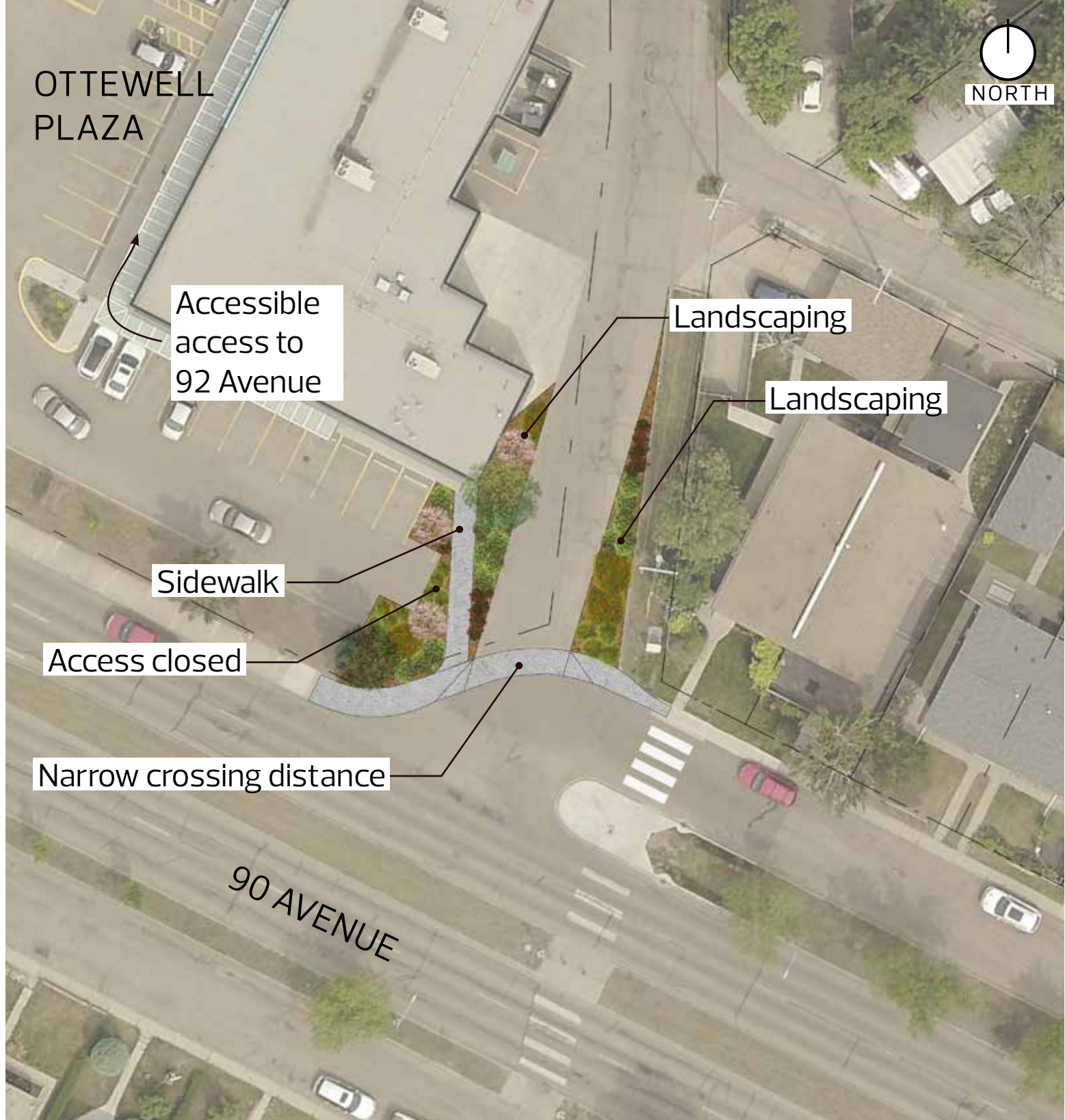
SOUTH ALLEY ACCESS
