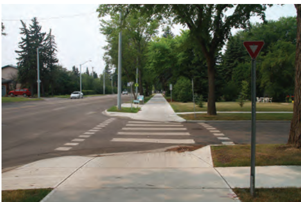
Figure 3.79: Crossride Treatment for use with shared pathway
