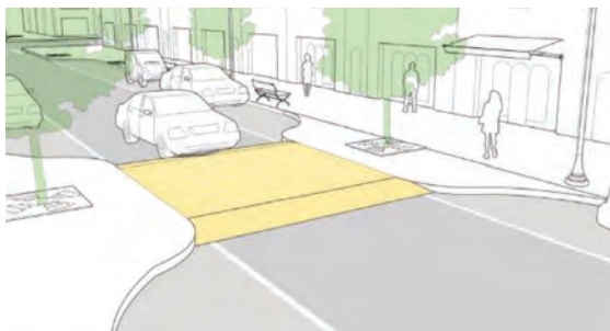
Figure 3.55: Raised Midblock Crossing 3
