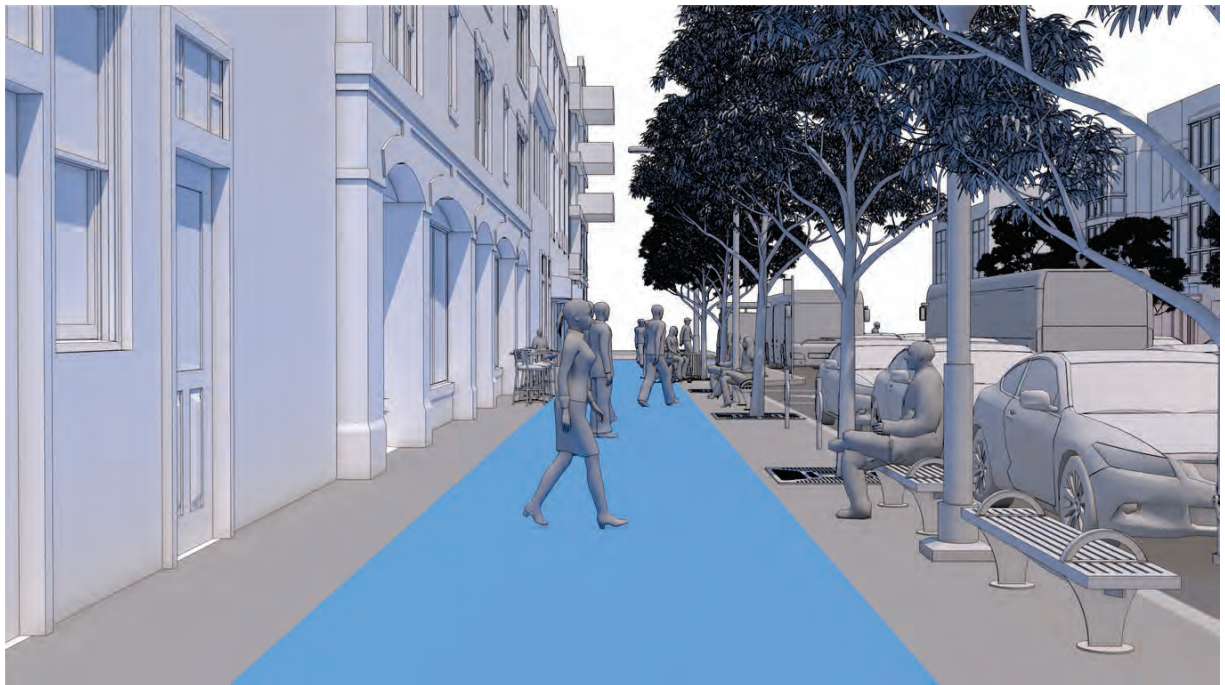
Figure 3.39 Pedestrian Through Zone
