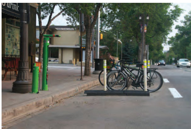
Figure 3.35 Bicycle Parking Corral in Ancillary Zone
