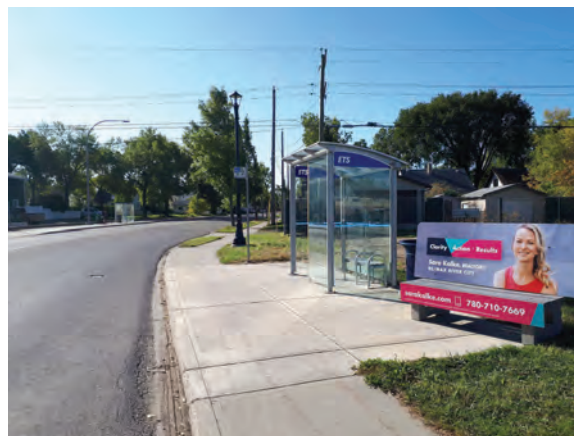
Figure 3.36 Transit Shelter (with sidewalk access and shelter oriented to protect waiting passengers from prevailing winds)
