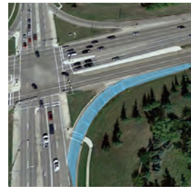
Low Exit Angle (Right Turn Channelization Free-Flow)
