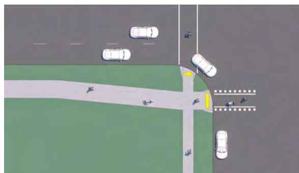
Figure 3.68: Intersection shared pathways Crossing (Bend-Out)
