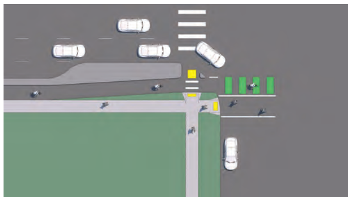
Figure 3.60: Protected Bicycle Signal Phase with Bend-In
