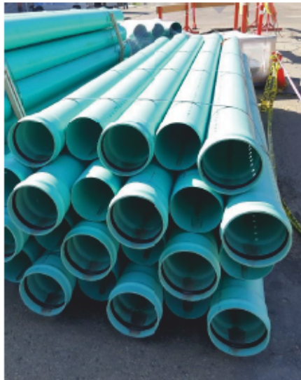
Photo 6: Perforated PVC Piping
