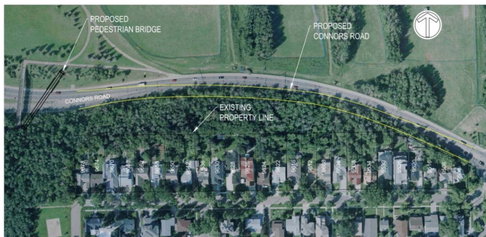
Figure 8. Option 2 - Partial Encroachment to South - Road Alignment
