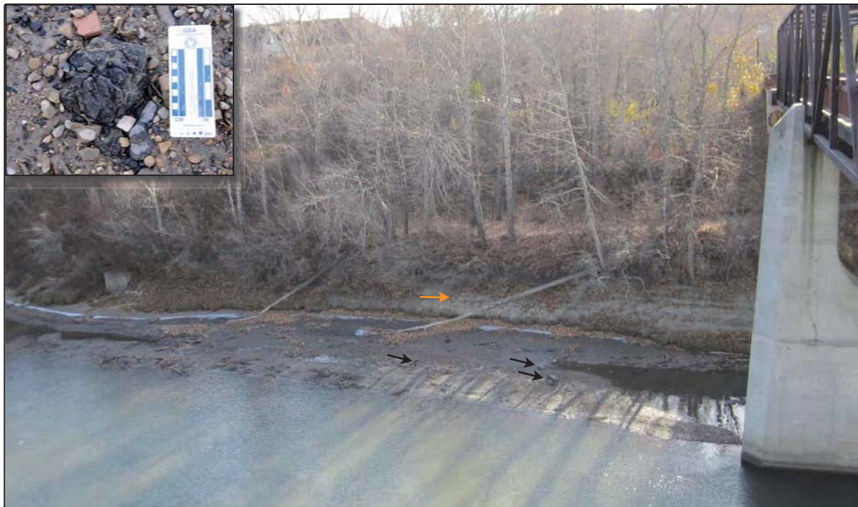
Figure 20. View looking southeast from footbridge observation deck showing exposed right (south) bank of North Saskatchewan River. Note thick floodplain deposits along bank (→) and reworked coal (inset) and bedrock fragments (→) along exposed river bed.
