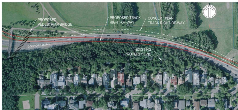
Figure 12. Option 3 - Full Encroachment to South - Track Alignment
