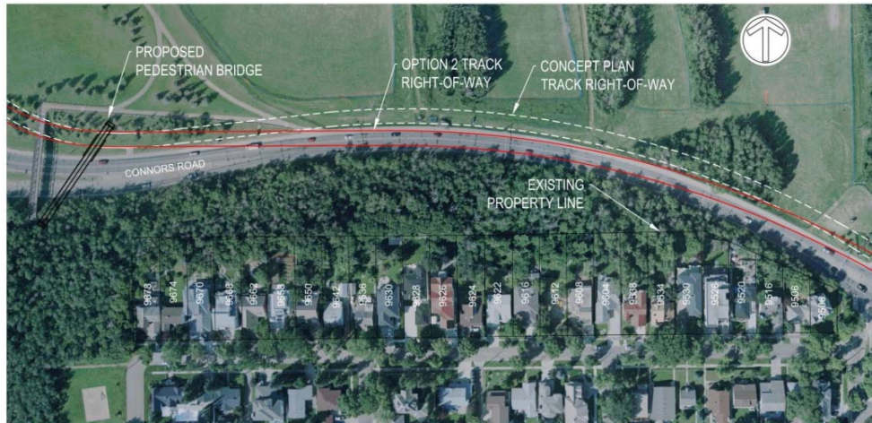
Figure 9. Option 2 - Partial Encroachment to South - Track Alignment
