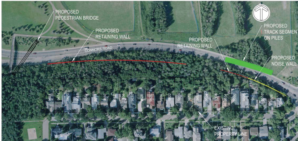
Figure 13. Option 3 - Full Encroachment to South – Structures
