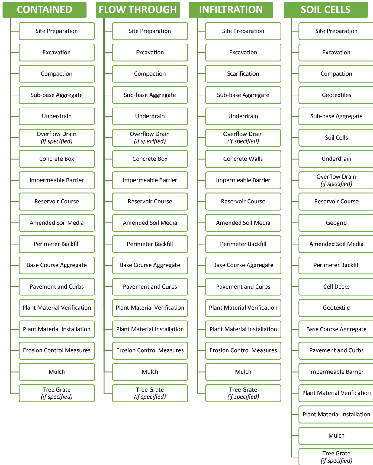
Figure 2. Construction Tasks by Box Planter Type
