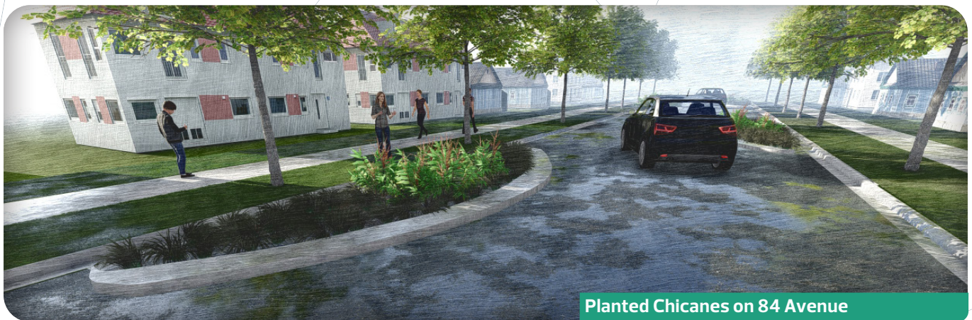
RAIN GARDEN PLANTINGS IN LANDSCAPED CHICANES ON 84 AVENUE
