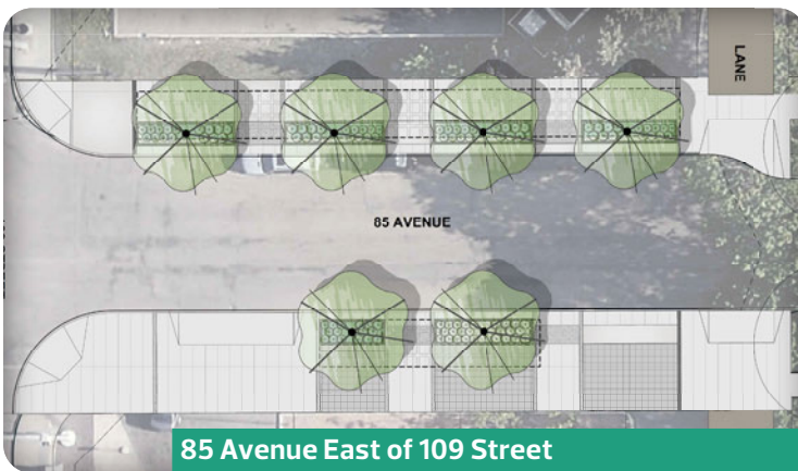
STRUCTURAL SOIL CELLS AND PLANTERS AT 85 AVENUE EAST OF 109 STREET
