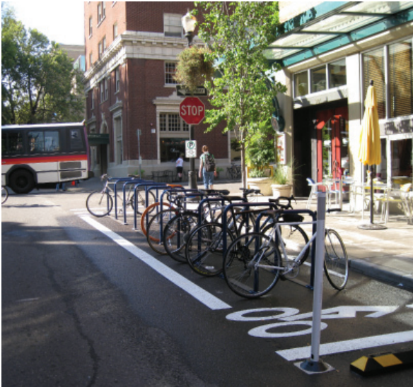
Figure 62: Bicycle Parking Curbside Parking Lane
