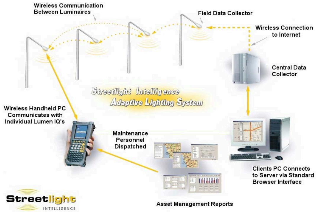
Figure 37 - Example Adaptive Lighting System
