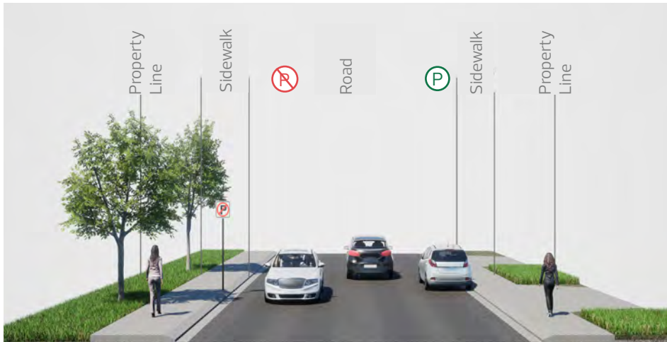
Scenario F : Sidewalks on both sides of the road. Trees planted on the ravine side of the road. Parking removed from one side of road
