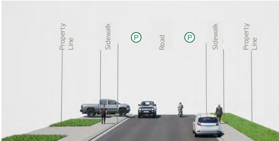
Scenario A: Sidewalks on both sides of the road with no boulevards. Parking unchanged.
