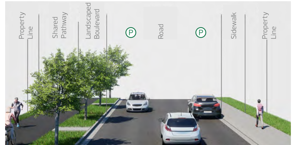
Scenario D: Shared pathway with landscape boulevard on one side of the road and a sidewalk without a boulevard on the other side. Parking unchanged.
