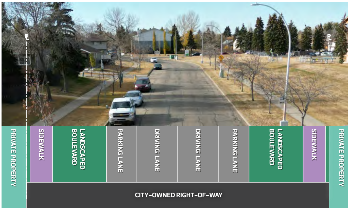
Existing Hooke Road cross section (looking west)
