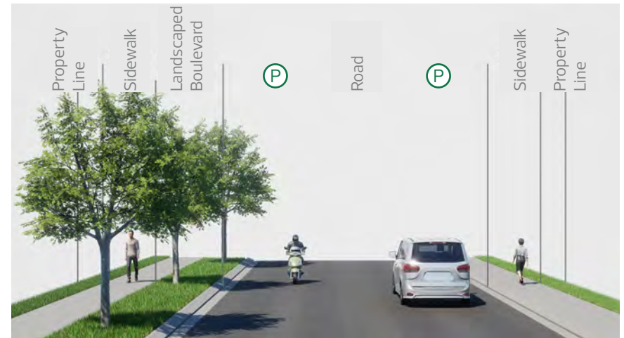
Scenario B: Sidewalk with a landscape boulevard on one side of the road and a sidewalk without a boulevard on the other side. Parking unchanged.
