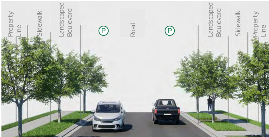
Scenario C: Sidewalks with landscape boulevards on both sides of the road. Parking unchanged.
