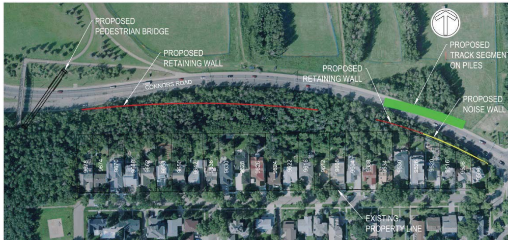
Figure 13. Option 3 - Full Encroachment to South – Structures
