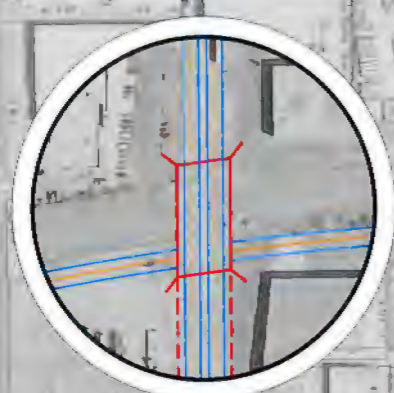
ALTERNATIVE B RUNNING PARALLEL TO RAIL UNDER STRUCTURE NO CONNECTION TO 149 STREET
